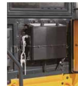
The **air conditioning filter** is easy to replace.
