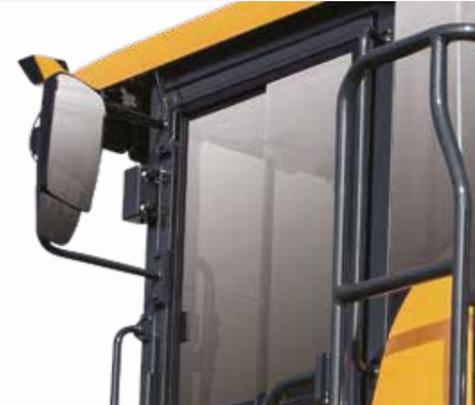
The **side mirror** is easy to adjust for optimal visibility and can be folded away to prevent damage during transportation.
