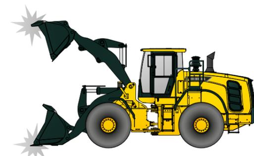
The **soft end stop** function reduces the hydraulic speed of the cylinder as it reaches the end of its stroke. This lessens the shock load of the stroke for increased operating comfort and better material retention.
