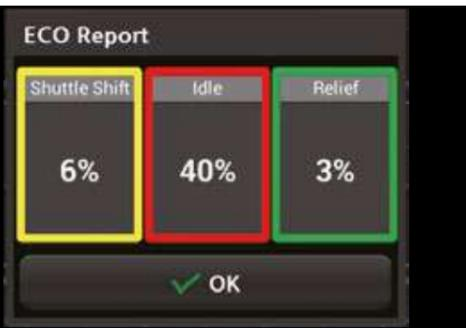
The **Eco Report** feature makes it easy for operators to develop efficient working habits by displaying real-time information about machine performance.
