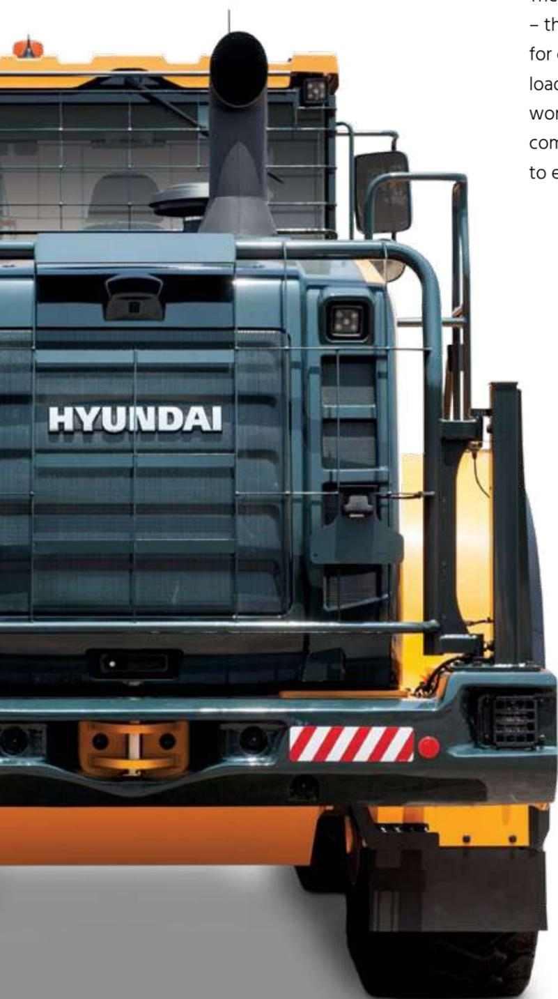
◀ A **rear grill guard** protects the engine hood, rear view camera, work lights and radiators from contact with any obstacles. The design does not impede the operator's view. The steel guard is hinged and opens to allow easy access to the radiator for cleaning or daily maintenance.
