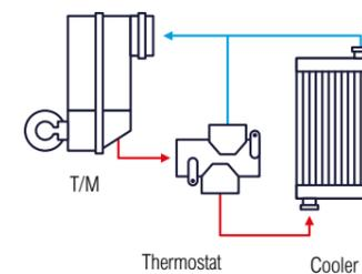
The HL960A is equipped with a **thermostat for transmission cooling**. This feature helps to warm up the fluid quickly and keeps it at the optimal working temperature, protecting components and increasing efficiency.
