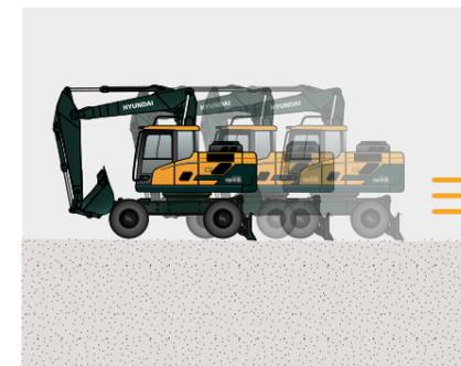
**Cruise control & speed limiter, creep speed drive**
