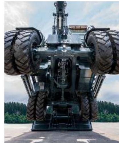
**Hydrostatic 4-wheel drive**
